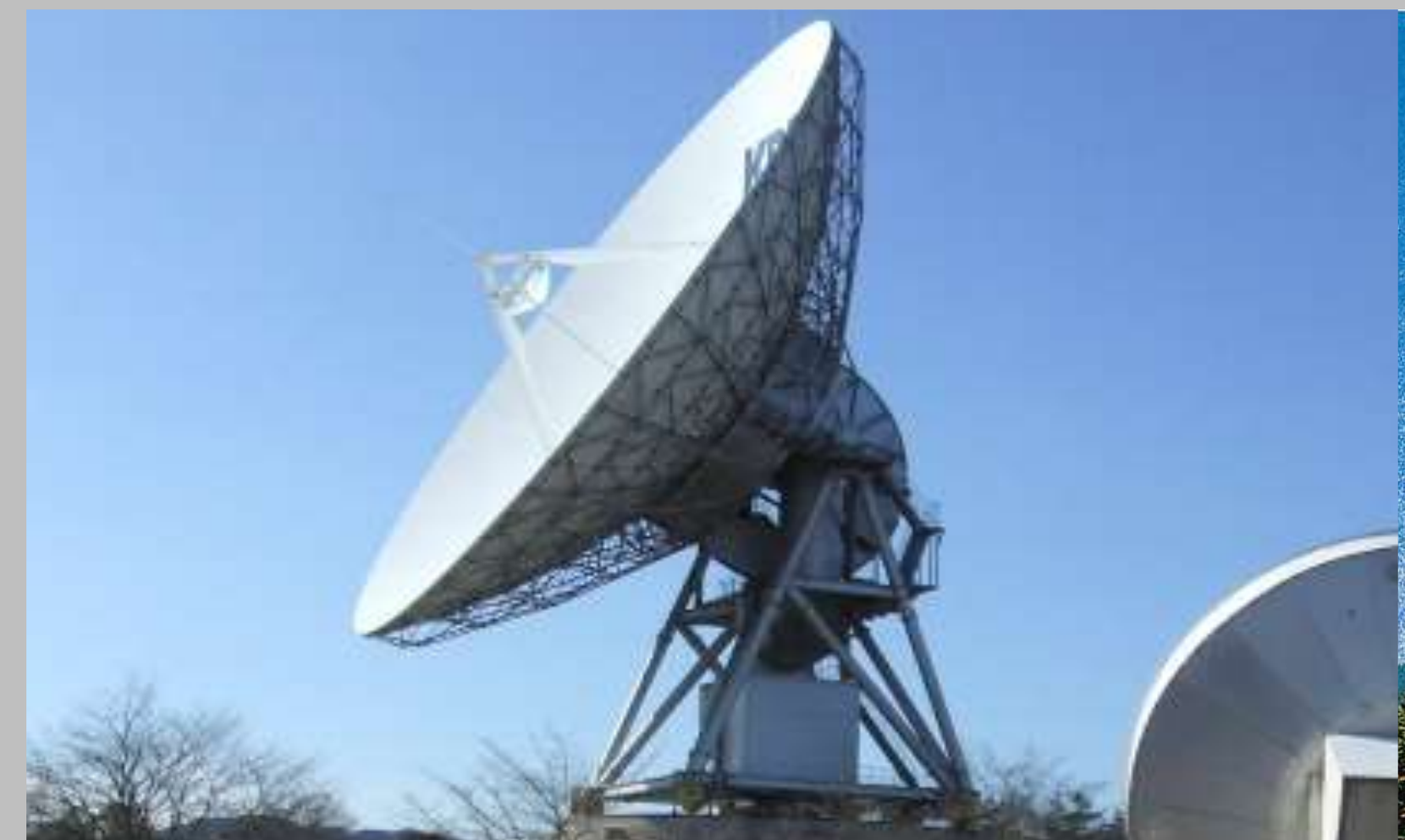
Intelsat standard-A antenna with 4 times beam feeding method
